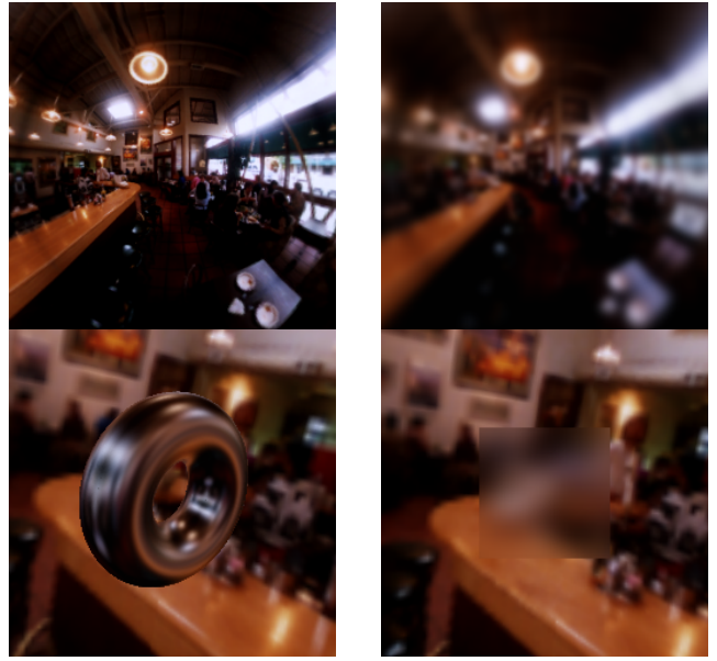
Figure 8: Top: original parabolic map used in this figure and Figure 7, as well as prefiltered map with a roughness of 0.01. Bottom: application of the filtered map to a reflective torus (left) and a transmissive rectangle (right).
