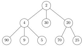
Suppose we have a heap containing at least two values. To remove and return its smallest element, while maintaining the heap property, we use the following function:
