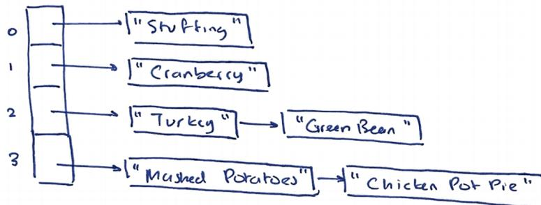
And this is the Hash Table after all strings have been inserted. Note that resizing is done by iterating through each chain bucket by bucket and recalculating the index that the string is inserted into.
