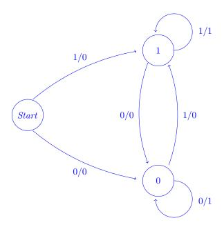
1.3 Write an FSM that will output a 1 if it recognizes the regex pattern  $\{10+1\}$ .
