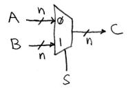
This mux has two n-bit inputs, A and B, and an n-bit output, C. Additionally, it has a special control signal labeled s, for *select*. The s signal is used to control which of the two input values is directed to the output. Specifically, the function of this mux can be described with these two rules:
