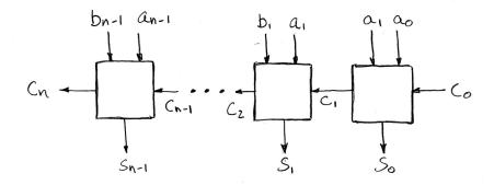
Inputs are applied at the top and after some delay, associated with the delay through the logic gates for the blocks, and the delay of the carry from stage to stage, the final result appears at the bottom.
