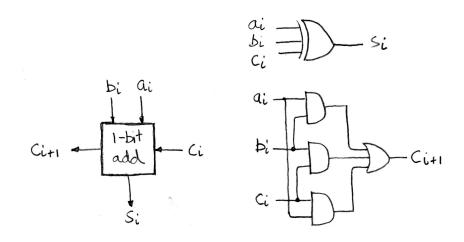
We will not bother creating a special block for the first column of the adder, because anything it can do the 1-bit adder block can do as well. We just need to figure out where to attach the carry-in to the first column. More on this later.
