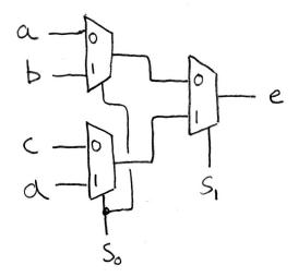
The first layer of muxes uses the  $s_0$  input to narrow the four inputs down to two, then the second layer uses  $s_1$  to choose the final output.
