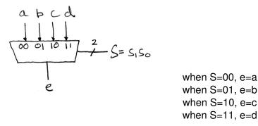
How would we come up with the circuit for this mux? We could start by enumerating the truthtable—in this case the function has 4 single bit data inputs and one 2-bit wide control input, for a total of 6 single bit inputs. The truth-table would have  $2^6$ , or 64 rows. Certainly, a feasible approach. If we where to do this, we would end up with the following logic equation:
