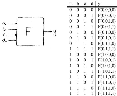
For each row of the table, the output column shows the output value of the block for the input pattern shown in the input columns.
