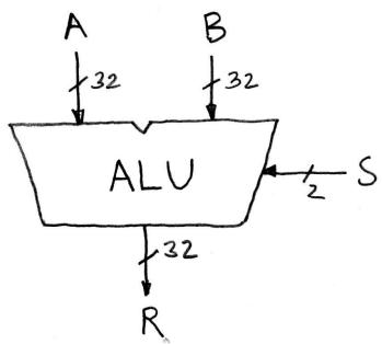
when S=00, R=A+B when S=01, R=A-B when S=10, R=A AND B when S=11, R=A OR B
