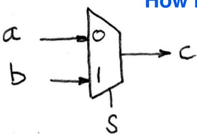
$$c = \overline{s}a\overline{b} + \overline{s}ab + s\overline{a}b + sab$$
