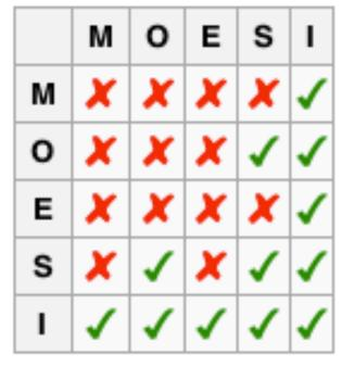
**Compatability Matrix**: Allowed states for a given cache block in any pair of caches
