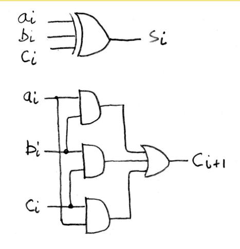
$$\begin{aligned} s_i &= \operatorname{XOR}(a_i, b_i, c_i) \\ c_{i+1} &= \operatorname{MAJ}(a_i, b_i, c_i) = a_i b_i + a_i c_i + b_i c_i \end{aligned}$$
