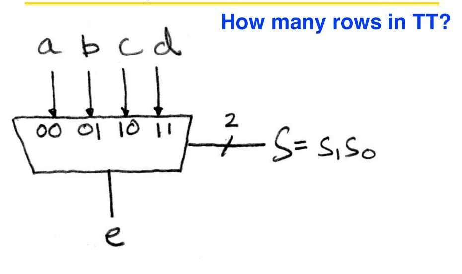
$e = \overline{s_1}\overline{s_0}a + \overline{s_1}s_0b + s_1\overline{s_0}c + s_1s_0d$
