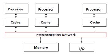
As seen in the figure above, the local caches communicate with each other via an *Interconnection Network*. Here we focus on snooping mechanisms, where this communication includes invalidation requests, monitoring of memory requests, and even transfer of data (cache blocks).
