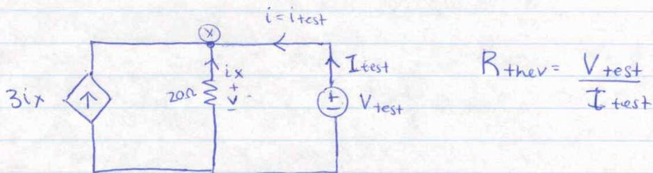
$V = V_{test}$  b/c they are in parallel
