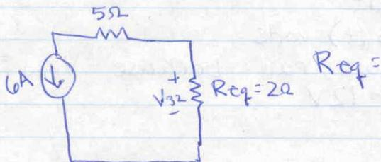
$$V_{32} = I R_{eq} = -6A \cdot 2\Omega = -12V$$
