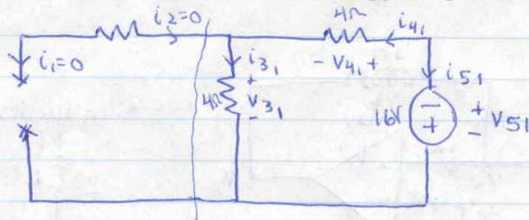
Voltage divider:  $V_{31} = \frac{-4}{4+4} \cdot 16 = -8V$
