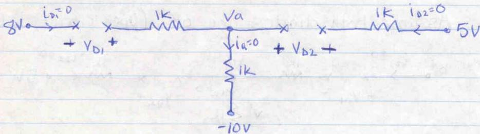
$$\left. \begin{aligned} V_{D1} &= -10\text{V} - 8\text{V} = -18\text{V} \\ V_{D2} &= -10\text{V} - 5\text{V} = -15\text{V} \end{aligned} \right\} < 0, \text{ our assumption was right.}$$
