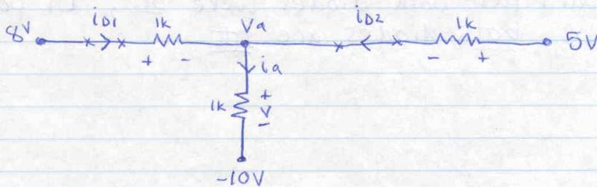
$$\text{KCL @ } V_a: i_{D1} + i_{D2} = i_a$$
