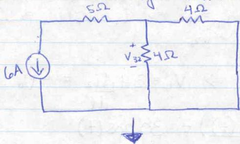
The  $4\Omega$  resistors are in parallel, therefore the voltage across them are the same, so we can find  $R_{eq}$
