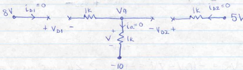
$$\left. \begin{aligned} V_{D1} &= 8V - (-10V) = 18V \\ V_{D2} &= 5V - (-10V) = 15V \end{aligned} \right\} > 0, \text{ so our assumption is wrong.}$$
