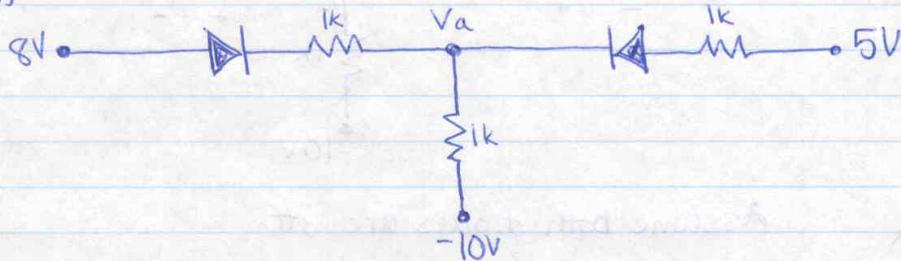
Assume both diodes are off. (Open circuit,  $i_D = 0$ ,  $V_D \leq 0$ )
