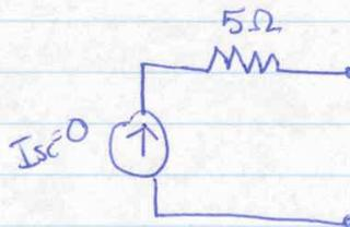
6) To find the Thevenin Equivalent, we must find  $V_{oc}$ .
