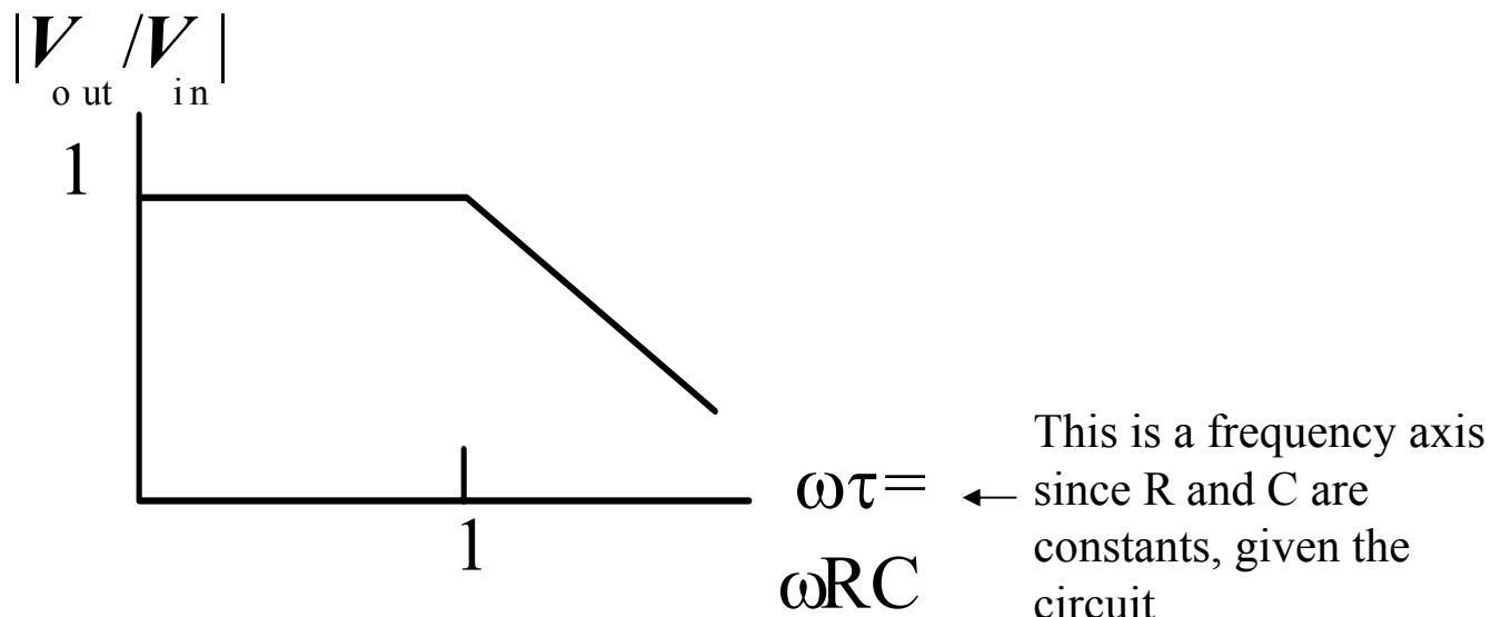
The plot shows that this is a **low-pass filter**. Its cutoff frequency is at the frequency  $\omega$  for which  $\omega RC = 1$ .
