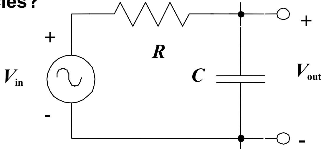
Assume the input voltage is  $v_{\text{in}}(t) = V_{\text{in}} \cos(\omega t)$  and represent it by the phasor  $\mathbf{V}_{\text{in}}$ . A phasor current  $\mathbf{I}$  flows clockwise in the circuit.
