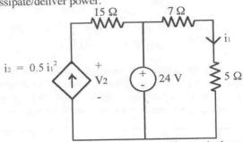
(b.) Let's ground the bottom node. The center node at the top is thus at 24V.
