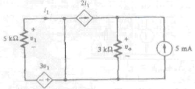
No dependent sources on the left:  $v_1 = 0 \text{ V}$ ;  $i_1 = 0 \text{ mA} \rightarrow v_0 = 3000(5 \text{ mA}) = 15 \text{ V}$
