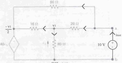
$$\frac{10 - v_1}{20} = \frac{v_1}{80} + \frac{v_1 - v_1/2}{16} \rightarrow v_1 = 3.2 \text{ V}$$
