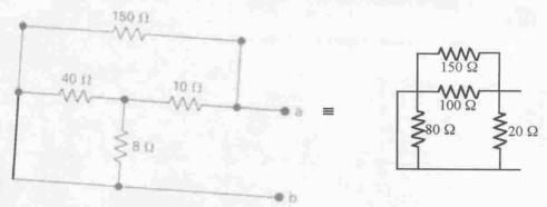
Because of the short circuit, the 80  $\Omega$  resistor is not seen. The equivalent resistance is: Req =  $20\|100\|150 = 15 \Omega$
