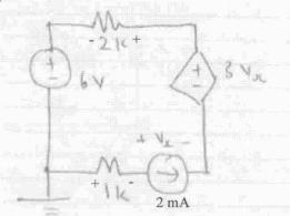
Doing KVL clockwise, starting at the ground:  $6 + 2000(.002) - 3v_x + v_x + 1000(.002) = 0$  $12 - 2v_x = 0 \rightarrow v_x = 6 \text{ V}$
