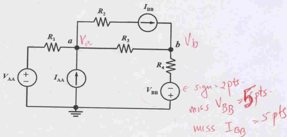
$$\frac{V_a - V_{AA}}{R_1} + \frac{V_a - V_b}{R_3} + I_{BB} = I_{AA}.$$
