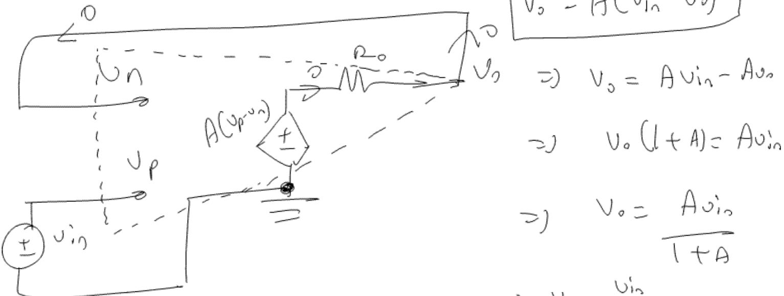
$$\Rightarrow V_o = A V_{in} - A V_o$$
