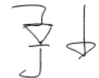
[Mechanical analog: check valve]
