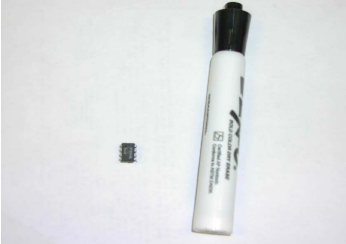
Figure 1. Comparing an op-amp IC to a whiteboard marker
