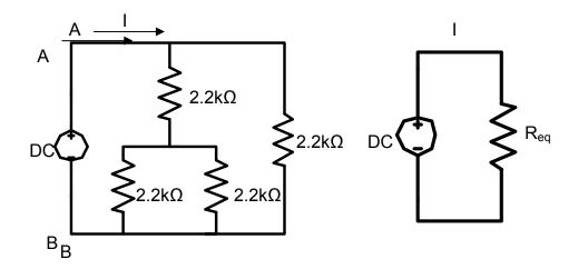
2) The three circuits given below are equivalent.
