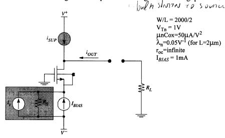
a) Draw the equivalent small signal circuit of this amplifier (10pts)
