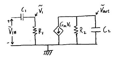
$$\frac{\widetilde{V_{out}}}{\widetilde{V_{in}}} = \frac{P_1}{P_1 + \frac{1}{jwC_1}} \left[ -G_m \cdot \left( P_2 | l \frac{1}{jwC_2} \right) \right] = -G_m P_2 \frac{jw P_1 C_1}{(l + jw P_1 C_1) (l + jw P_2 C_2)}$$
