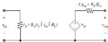
Note 1: both the input and the output resistances depend on the load and source resistances, respectively (note typo in Fig. 8.47 in text)
