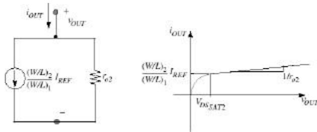
The model is only valid for  $v_{DS} = v_{OUT} > v_{DS(SAT)} = V_{GS} - V_{Tn}$
