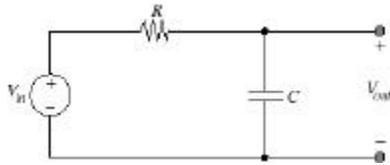
Replacing the capacitor by its impedance,  $1/(j\omega C)$ , we can solve for the ratio of the phasors  $V_{out}/V_{in}$
