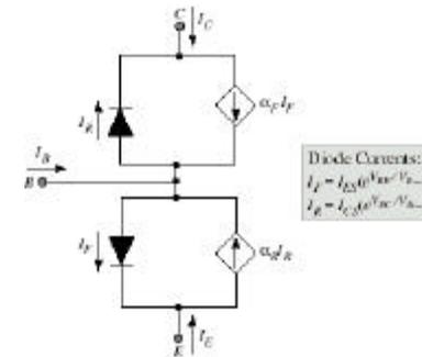
This model for the BJT applies to general device structures, with the four parameters  $I_{ES}$ ,  $I_{CS}$ ,  $\alpha_F$ , and  $\alpha_R$  being linked by “reciprocity”
