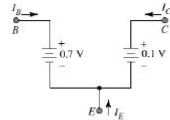
note that the batteries make the controlled current sources irrelevant to the circuit.
