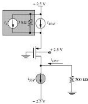
Small-signal model is identical to n-channel version
