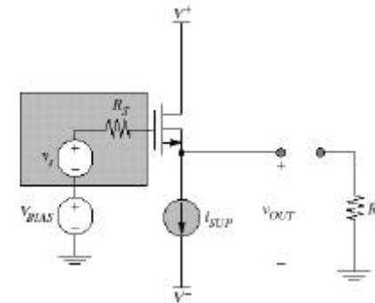
For DC bias, neglect small signal source (and its resistance) and the small-signal load resistance;  $i_{SUP} = I_{SUP}$
