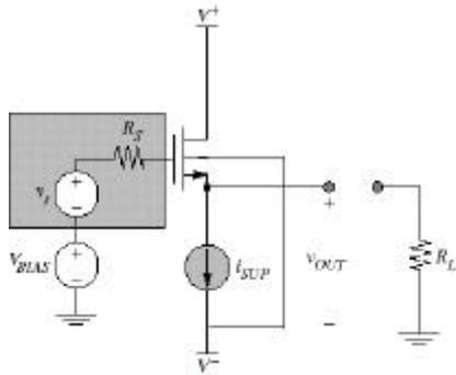
The threshold voltage  $V_{Tn}$  is not a constant, since the source-bulk voltage  $V_{SB}$  increases as  $V_{OUT}$  increases:
