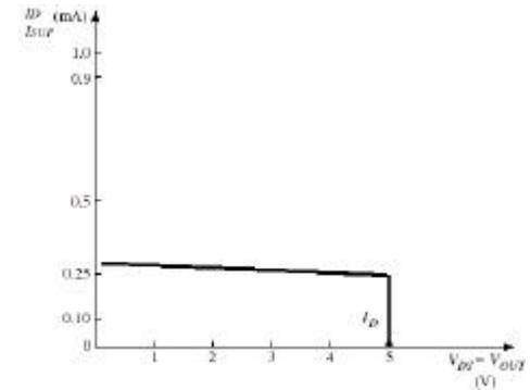
The region of input bias voltage  $V_{BIAS}$  for which the current source and the MOSFET are in their constant-current regions is *extremely* small ....
