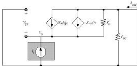
Analysis:  $i_{out} = i_d$  and  $i_d = -i_g - i_s = -i_s = -i_t$
