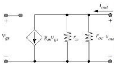
Tradeoffs are different from case of resistor load since  $I_D$  is now decoupled from the small-signal current supply resistance  $r_{oc}$
