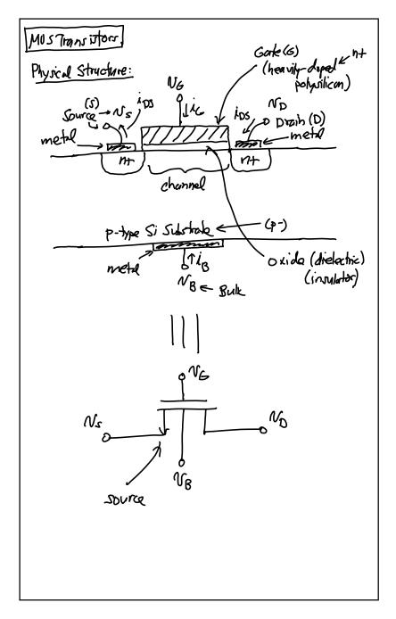
NMOS Transistor Morthematical Model
