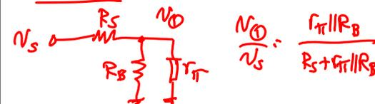
$$\frac{v_o}{v_s} = \frac{r_{\pi} \| R_B}{R_S + r_{\pi} \| R_B}$$
