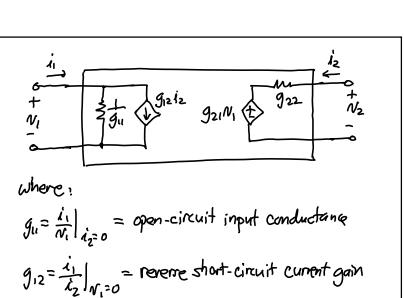
$g_{zz} = \frac{N_z}{i_2} \Big|_{M=0} = Short-ciruit output resistance$ Assuming a derign to amplify in the forward direction - neglect the current source giziz in the
