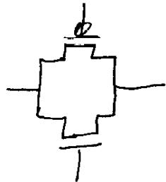
the n-channel can "pass" anything from  $0V$  to  $V_{DD} - V_{tn}$ . The p-channel can pass  $-V_{tp}$  to  $V_{DD}$ . You need both to pass  $0$  to  $V_{DD}$ .
