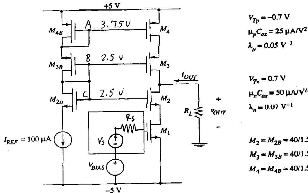
A CMOS cascode transconductance amplifier and the device data are shown above. There is no backgate effect.
