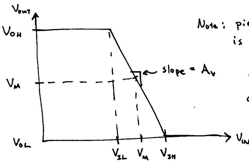
Note: piecewise linear approximation is ok for CMOS inverter.
