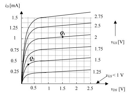
(a) [4 pts.] What is the small-signal transconductance  $g_m$  at the operating point  $Q_1$  in mS? You can find the answer either from the drain current equations or graphically: in either case, be sure to explain your method clearly.
