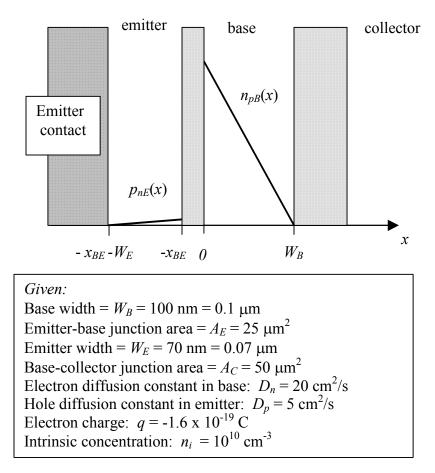
(a) [4 pts.] The collector current for this forward-active npn bipolar transistor is  $I_C = 20 \ \mu$ A. From the cross section of the device shown above, find the numerical value of the minority electron concentration at x = 0, at the base side of the emitter-base depletion region.
