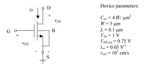
An improved model for the velocity-saturated MOSFET is:
