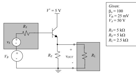
(a) [3 pts.] Find the numerical value of  $V_B$  such that  $V_{OUT} = 2.5$  V. Your answer should be accurate to +/- 5%. Notes: (i) the gray boxes indicate small-signal elements that can be neglected for the DC bias analysis and (ii) the DC base current  $I_B$  of the bipolar transistor can be neglected for the bias solution.
