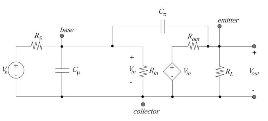
Find Miller capacitor for  $C_{\pi}$  -- note that the base-emitter capacitor is Between the input and output
