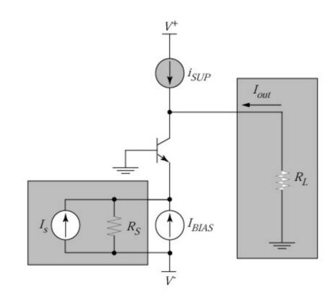
Same procedure: start with two-port model and capacitors
