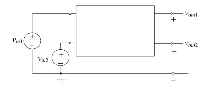
$$v_{out,diff} = A_{v,diff} (v_{in,diff}) = A_{v,diff} (v_{in1} - v_{in2}) \dots \text{ large}$$
