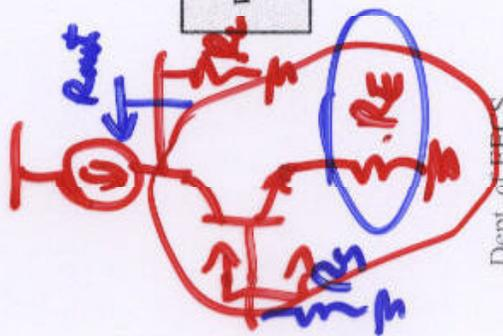
$\frac{v_o}{v_i} = \frac{v_o}{v_{\pi}(1 + g_m R_E)}$
