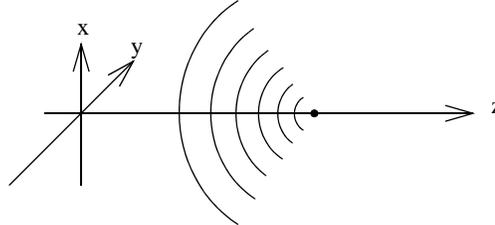
At a given  $z$ -plane, the spherical wave has constant phase around circles. The form of the spherical wave is  $\cos\left[-\frac{k(x^2 + y^2)}{2z_0}\right]$  for a spherical wave converging to the point  $z_0$  on the axis. A lens modifies the wave front, for example from planar to spherical.
