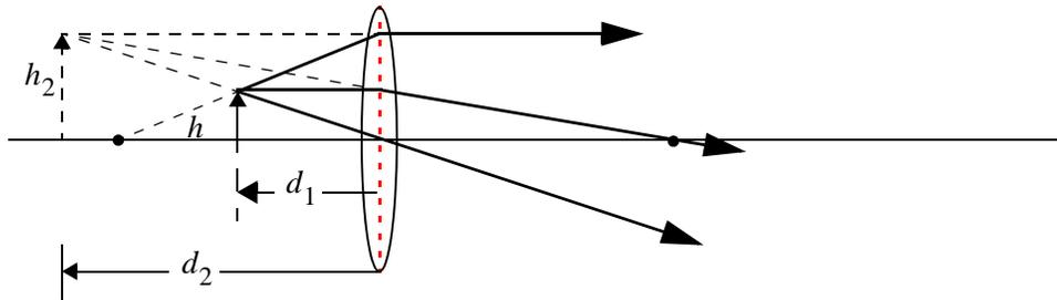
The light emerging from the lens appears to be coming from the object with height  $h_1$  at distance  $d_2$  behind the lens.
