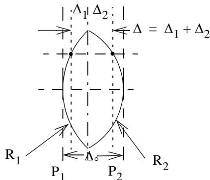
In propagating from plane  $P_1$  to  $P_2$ , the light travels a distance  $\Delta = \Delta_1 + \Delta_2$  in the glass and a distance  $\Delta_0 - \Delta$  in air, where  $\Delta_0$  is the thickness at the thickest part of the lens. The phase delay depends on  $(x, y)$ :
