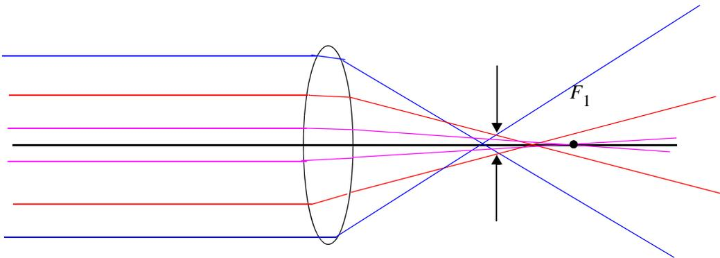
Rays toward the edge of the pupil (even parallel to the axis) violate the paraxial condition on the incidence angle at the first surface. They focus closer (for biconvex lens) than  $F_1$ . No truly sharp focus occurs. The least blurred spot (smallest disc) is called circle of least confusion, or best focus. This form of symmetric aberration is spherical aberration.
