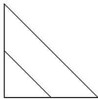
right angle prism with a roof on hypotenuse
