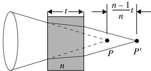
A simple calculation based on the paraxial approximation shows that the focus is displaced by amount . However, at steeper incidence angles, the focal shift becomes a function of the incidence angle, which leads to spherical aberration.
