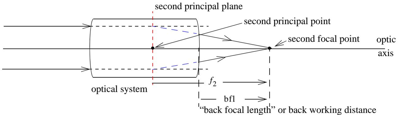
Now, we take the rays entering the system and those emerging from the system and extend them. They intersect on a plane called the “Second principal plane”. Similarly, the first focus and “first principal plane” are defined for rays emerging from the system parallel to the axis, which all emanate from a point.
