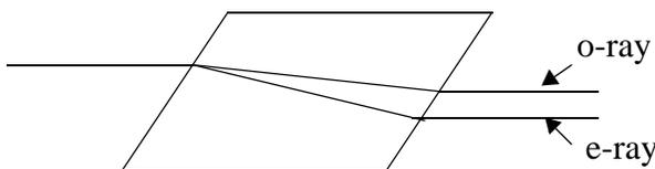
Common birefringent crystals-quartz ( $\text{SiO}_2$ ), calcite ( $\text{CaCO}_3$ )
