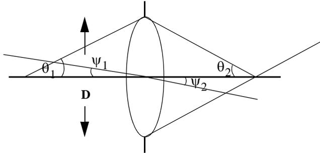
Due to diffraction at the aperture stop, the image of a point is slightly blurred. Diffraction theory tells us that the image depends on the shape of the aperture. For a circular aperture:
