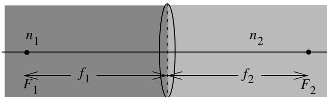
The front and back focal lengths are not the same in this case
