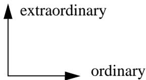
The ordinary component has index  $n_o$  and the extraordinary component has index  $n_e$ . As propagation direction varies the ordinary component always has index  $n_o$  but  $n_e$  varies between  $n_o$  and  $n_{e0}$ .
