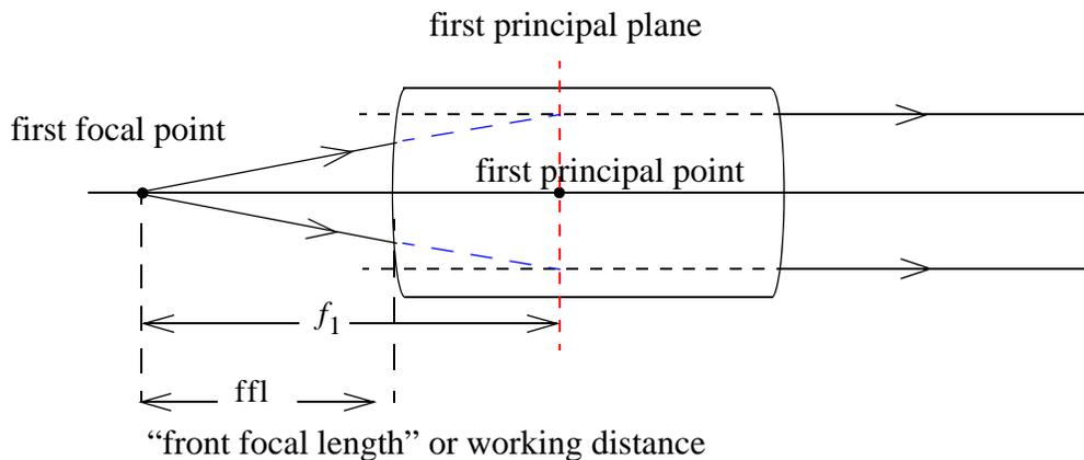
We define  $f_2$  as the distance from the second principal plane to the second focal point. Similarly we define  $f_1$  as the distance from the first principal plane to the first focal point. For a system immersed in air (same index on both sides),  $f_1 = f_2$ .
