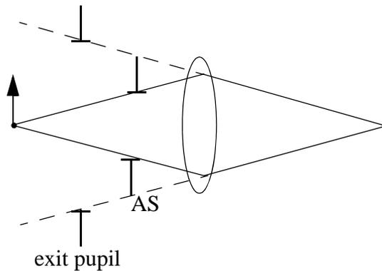
The exit pupil defines the cone angle of light converging to the image point. Later, we will see that this is important in determining the image resolution that is set by diffraction.
