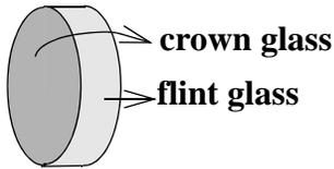
The 'D' wavelength, near the center of visual brightness curve is chosen as the nominal wavelength for specifying focal length. We then choose 2 indices on either side, for achromatization, for example, 'C', and 'F'.
