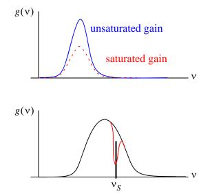
*homogeneous broadening*: Under saturation, entire gain curve is reduced. Shape is unchanged
