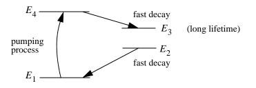
Due to long lifetime in level 3, population stacks up. Any atoms in level 2 rapidly drop back to level 1.
