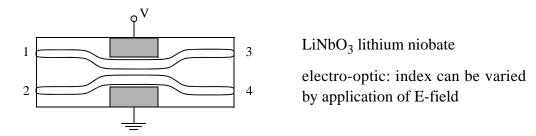
By manipulating the voltage input, 1 can be routed to 3 or 4. Similarly for input 2.
