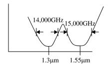
Dense WDM (DWDM) wavelength channels ~ 1nm separation.
