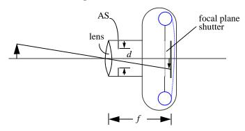
The aperture stop (AS) is variable to control the amount of light reaching the film. By convention, the AS is normalized to the lens focal length to give a dimensionless parameter called *F number* or *F-stop*
