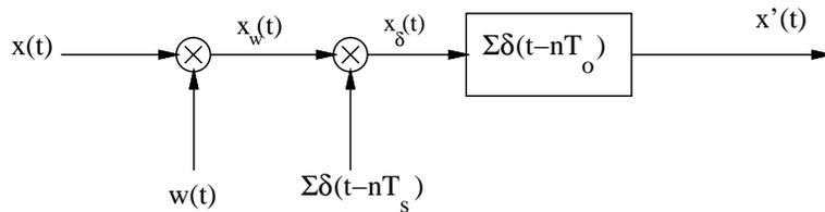
Figure 1: Window, sample in time, sample in frequency (DFT)
