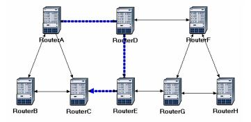
4. Repeat step 2 to show the route for the traffic demand between **RouterB** and **RouterH**. The route is as shown below. (*Note:* Depending on the order in which you created the network topology, the other "equal-cost" path can be used, that is, the *RouterB-RouterA-RouterD-RouterF-RouterH* path).
