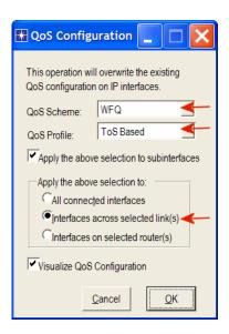
*Note:* Since the **Visualize QoS Configuration** radio button is checked, the link is colored based on the QoS scheme used (green for WFQ).
