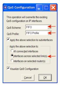
*Note:* Since the **Visualize QoS Configuration** radio button is checked, the link is colored based on the QoS scheme used (blue for FIFO).
