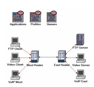
The QoS Attribute Config node defines attribute configuration details for protocols supported at the IP layer. These specifications can be referenced by the individual nodes using symbolic names. It defines different queuing profiles such as FIFO, WFQ, priority queuing, custom queuing, MWRR, MDRR, and DWRR.
