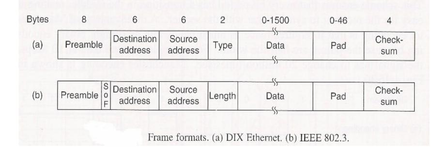
• 8 byte preamble (DIX Ethernet): alternating 1/0 combination producing 10Mhz square wave [@ 10Mbps] for 6.4  $\mu sec$ ; used for receiver synchronization
