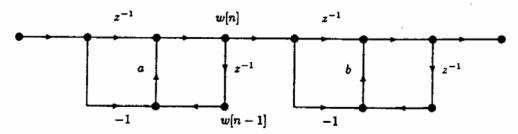
The first delay in the second section has output w[n-1] so we can combine with the second delay of the first section.
