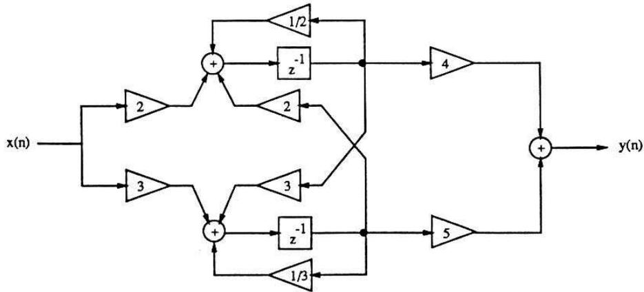
6. Find the transfer function of the system shown in the figure above.
