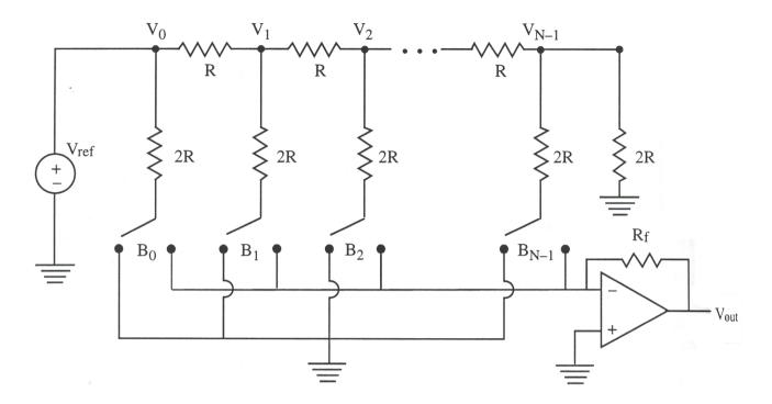
The switches are transistors, where the  $B_i$  control whether the transistors conduct to ground (left position,  $B_i = 0$ ) or to the op amp (right position,  $B_i = 1$ ). The op amp then adds all signals input to its minus terminal, with a weighting determined by the resistor values. To find the exact relationship between  $V_{out}$  and the  $B_i$ , first apply KCL at Node N-1 at the upper right, to give:
