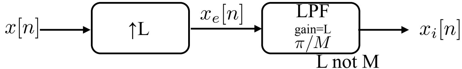
$$\begin{aligned} X_e(e^{j\omega}) &= \sum_{n=-\infty}^{\infty} \underbrace{x_e[n]}_{\neq 0 \text{ only for } n=mL \text{ (integer } m)} e^{-j\omega n} \\ &= \sum_{m=-\infty}^{\infty} \underbrace{x_e[mL]}_{=x[m]} e^{-j\omega mL} = X(e^{j\omega L}) \end{aligned}$$
