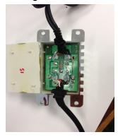
4) Unsolder the leads to Female RCA cables on GLI to remove it.
