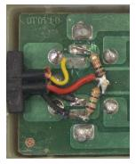
7) Lift the top\* wire (typically white or orange) on the left hand end of the circuit, and put in a resistor divider circuit:
