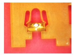
12) The above mounting platform was laser cut from inexpensive cast acrylic, the kind labeled "Chemcast" in red diagonal printing from TAP Plastics. Extruded acrylic (and some more expensive cast acrylic) did not hold finer details of flexural fingers (shown to right of platform) designed to hold nuts in place during insertion of their bolts.
