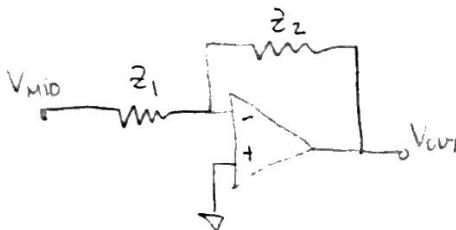
$$\text{From above, we have } V_{MID} = V_{IN} \left( \frac{R_3}{R_3 + C_2 R_1 R_3 s + R_1} \right)$$
