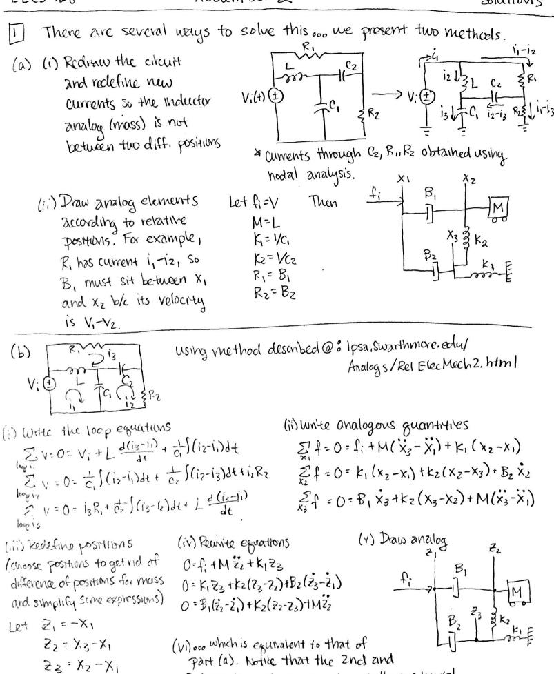
3rd equations give you everything in the mechanical Circuit except for force, and the 1st equation connects all the "appendages" to the loop corresponding to the original node @ Vi.
