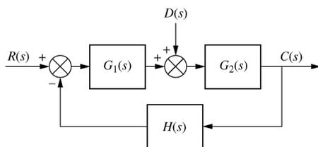
Fig. 1. Control System Block Diagram.
