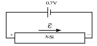
$E_c$  and  $E_v$  vary in the opposite direction from the voltage. That is,  $E_c$  and  $E_v$  are higher where the voltage is lower.
