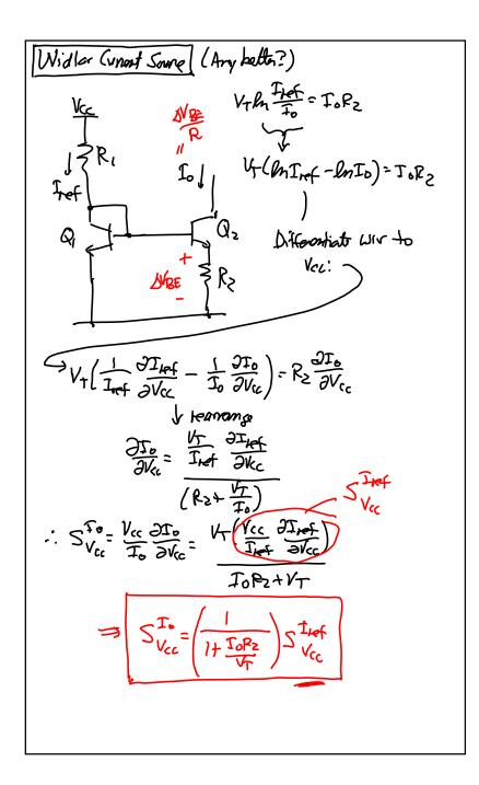
Since Fref= VCC-VBE(A) = VCC = SV. ~1  $\therefore \left| S_{V_{cl}}^{T_{o}} = \frac{1}{1 + \frac{\Gamma_{o}R_{c}}{1 + \frac{\Gamma_{o}R_{c$ For Inf ImA. Is= 10, 1A, R2= 11.9KD, then 107, sin Ver -> 1.390 A in I. (bathen than a simple current snurre) How can we do better? -> UK anothe netting reforme 1 V (D VBEIA) → bcp emith junction voltage ② V2→ Zenerdiodo (3) V<sub>1</sub> → theshold place (MOS) V () V\_7= kT -> thermonology () + √ ⑤ Eg → bandgap
