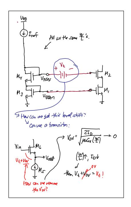
EE 140/240A: Analog Integrated Circuits Lecture 11w: High Swing Current Sources
