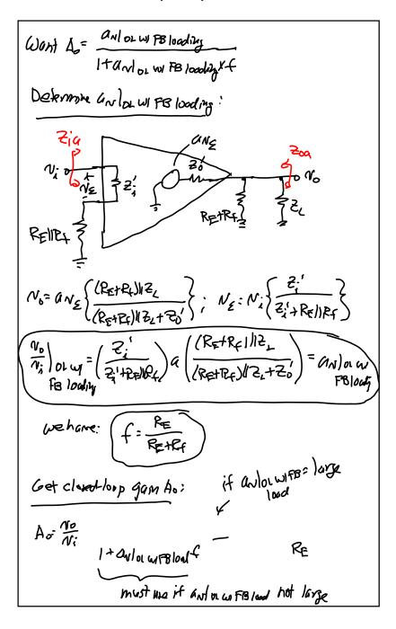
What about 2; {Zo? => For the open-loop op amp wit FB localing. Zia= Zi+RE//RC 2 Open-loop cmg, Zoa= Zóll(RE+RF)/17L 5 4 FB loaching = For closed-loop, just multiply on druide by (Hart) depends on the type of FB connection Sever: Zi=Ziu (Itavf)=(Zi+Re)/Rf)(Itavf) Shunt: 20: ZoalowFB 20'ILRETRY) ILRE 17GVILLWFBF 1+ 4NOLWFRXF What about W-3018? (-30B) cloved-loop = [W-30B] OL W/ Fr3] × (I+and with the cloved-loop)
