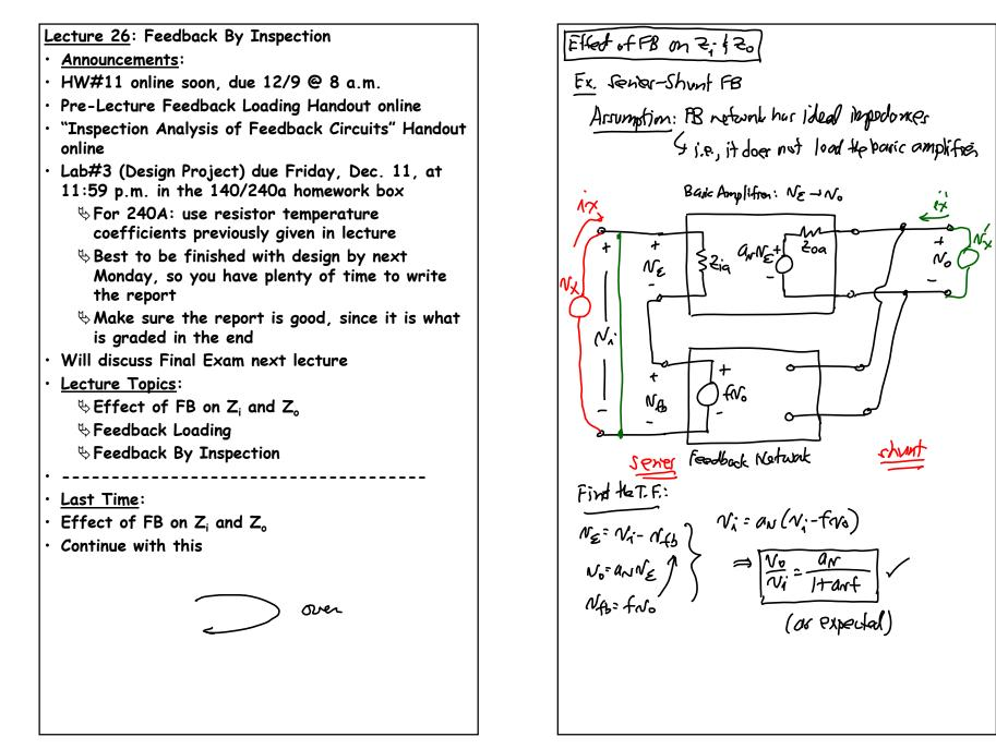
Find z: - - - : logo gar NX=NE+NG = NE+ fro= NE+ fan Ns= Vs ( Itanf. 1x= NE 2:0 closed loop part impodence  $Z_n = \frac{V_{x}}{i_{x}} = \frac{V_{x}(1+\alpha_{n}f)}{\frac{V_{x}}{2i_{n}}} = \frac{2i_{n}(1+\alpha_{n}f)}{\frac{1}{2i_{n}}} = \frac{2i_{n}}{\frac{1}{2i_{n}}}$ orignel Open-lop impadure of op amp When use service } Classed loop imput impedance Connection @ mpdf } raised by (it and)? If Zit → betty notion \ amplifia! at least it accept a Notige input better
